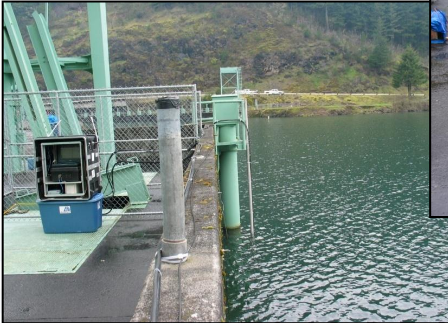
Surface electronics for data storage and echosounder control
