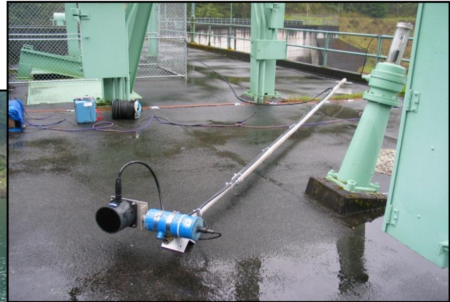
Pole-mounted BioSonics transducer and rotator assembly
