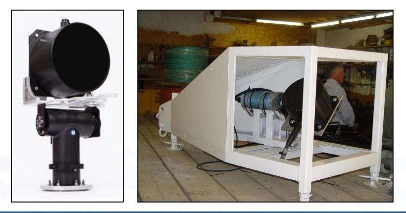
Split beam transducer/rotator assembly was lowered onto the river bed from work boat
