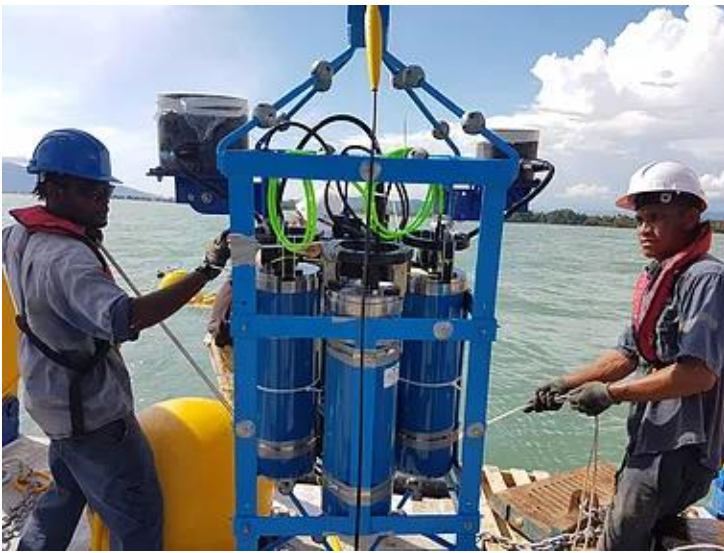
Custom mooring frame for DT-X SUB and battery packs prepared for deployment aboard ship in Papua New Guinea
