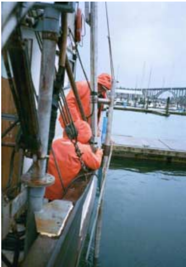
Figure 4. Installation of the hydroacoustic transducer mount aboard the F/V Orca.
